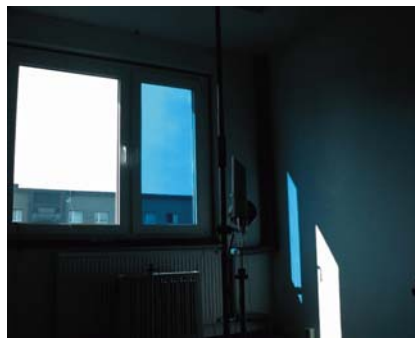
Figure 11 Office room with electrochromic windows: real picture. 22 nd September 2005 at 2 p.m., clear sky; left window bleached, right window coloured
