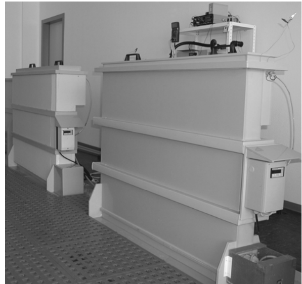
Fig. 1 Wet processors for electrodeposition of electrochromic films on glass panes up to 1 sqm.
